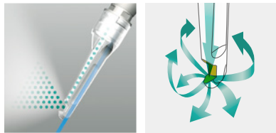
Direction of powder injection
